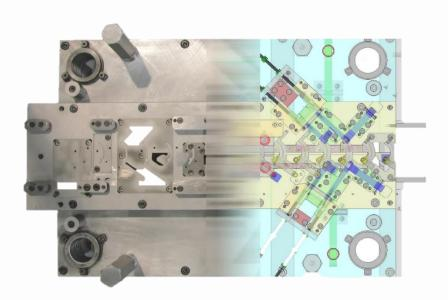
The **design of dies** and **automatic assembly machines**, as well as the mechanical design of innovative projects, is carried out entirely in-house by our technical department equipped with a 3D CAD system. We are able to acquire customer drawing files to speed up the design process; construction is entrusted to our tooling department.
